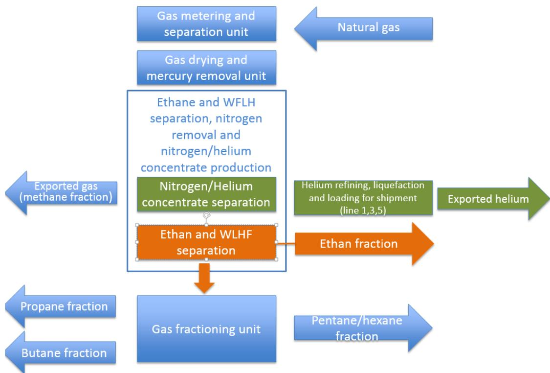
**Figure 2.2: Natural gas processing flowchart**
