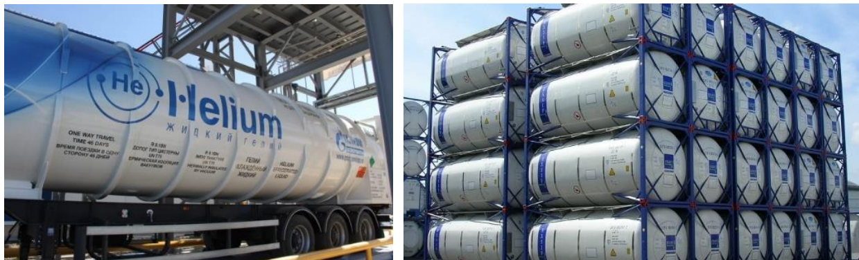
Figure 5.10 Isothermal tanks for transporting the liquefied helium 16
